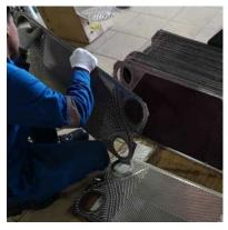
DYE PENETRANT TEST
